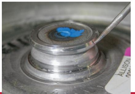
The edges of a new torque converter are clearly in better condition for longer life.
