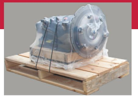
Our transmissions use specially-designed pallets to protect the transmission. Note that no weight is borne by the oil pan.
