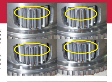
Their transmission rear carrier gear shaft has a shim ring added to compensate for wear instead of using an Allison-approved one-piece sleeve.
